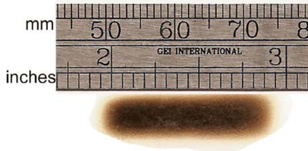
Figure 9-14 Typical Raw Beam Profile of COMPexPro® Laser
