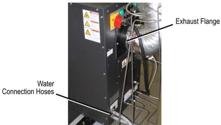
Figure 5-9. Water Connections on the Laser
