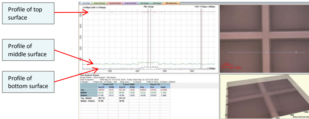
Fig. 91. Step height measurement on unfiltered image
